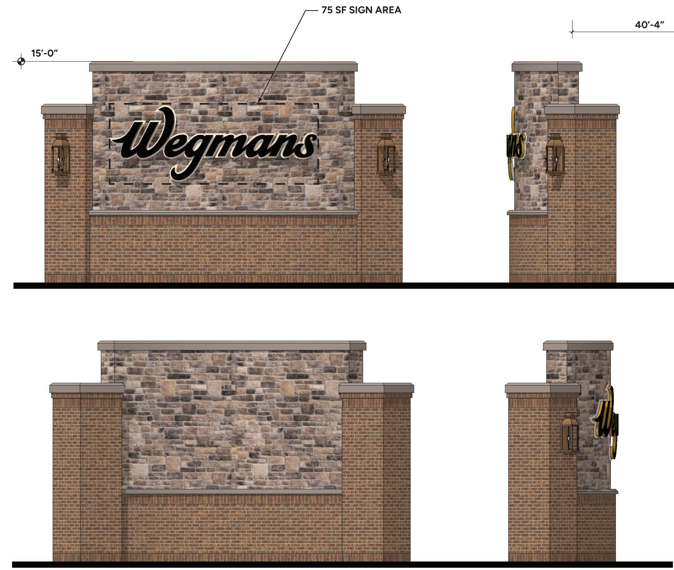
Monument Sign Elevations Scale: 1/4"=1'-0"
